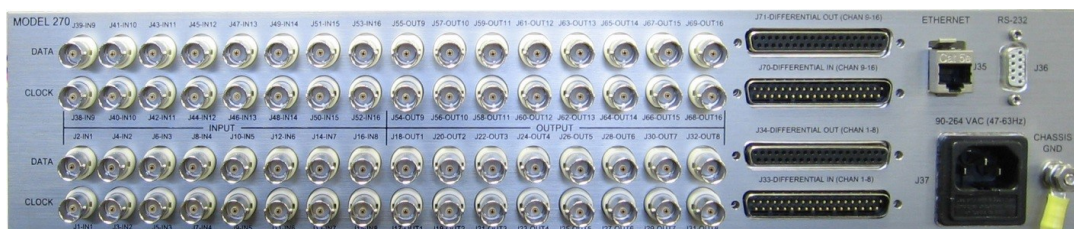
Rear Panel 16 Channel Unit
