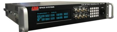
**Model 44XX** Telemetry Receiver products support BSS output with encapsulated quality (DQE). The Data / Quality information can then be transported to a BSS unit via Data/Clock or Ethernet and used in the BSS algorithms.
