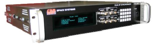
The Model 2265EC is capable of maintaining synchronization with the signal of interest down to  $-3$  dB Eb/No at signal levels as low as 100mVp-p. When searching for the signal, acquisition is attainable in less than 50 bits. The unit can maintain synchronization for a period of at least 256 bit periods without a transition.
